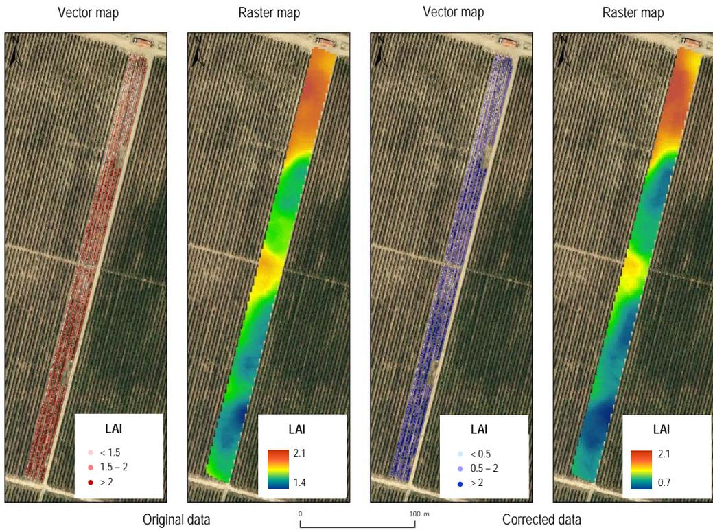
**Fig. 4. Vector and raster maps of LAI using original data (left) and corrected data (right) from LiDAR sensor.**
