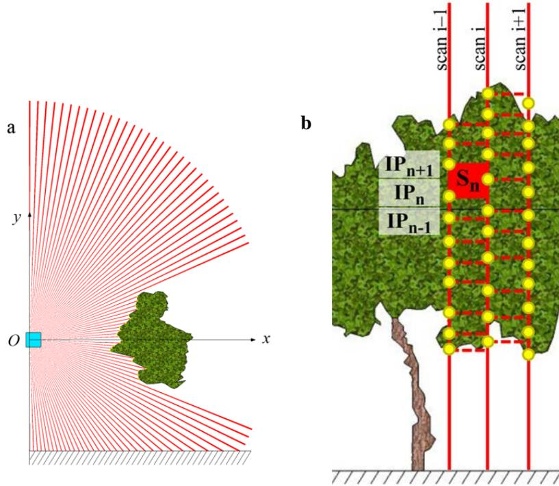
**Fig. 2. a) Coordinate system of the sensor for a complete single scan (0° to 180°). b) Intercepted points (IP) generated by three consecutive scans, and surfaces assigned to each point ( $S_n$ ).**
