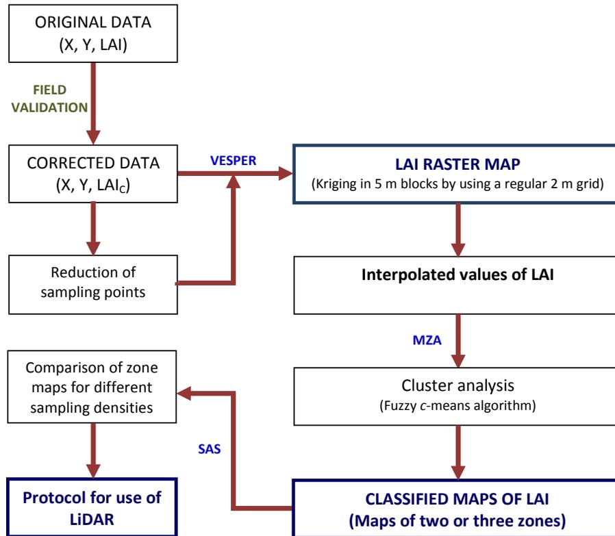
**Fig. 3. LiDAR assessment method to obtain LAI maps in vineyard.**
