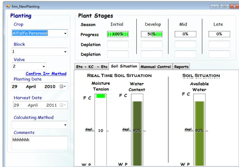
**Figure 1.** The main system operation control screen, showing the crop type, the current planting stage, Irrigation scheduling, soil situation monitoring, manual control and reporting tabs.
