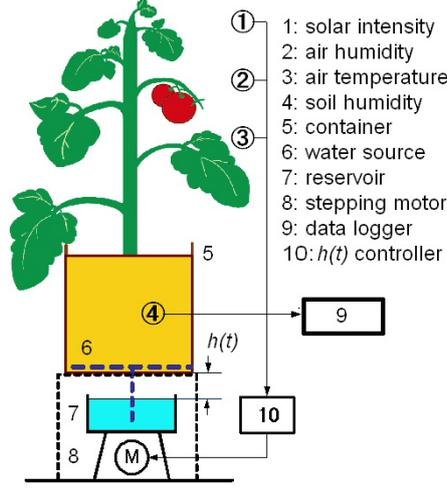
Fig. 1. Experimental setup for the adaptive irrigation control
