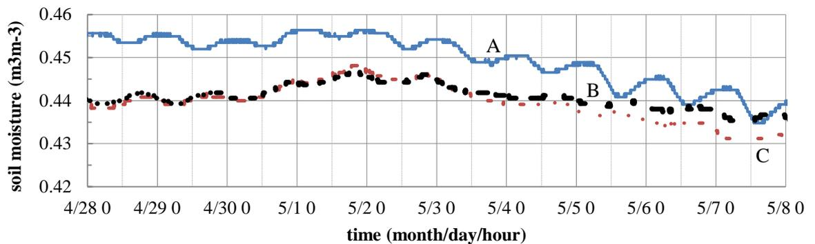
Fig. 4 Time variation of soil moisture at each point under proportional action.
