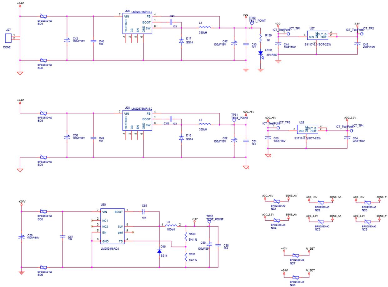
Figure 2. Circuit diagram of the power division part (24V, 12V, 5V, 3.3V).
