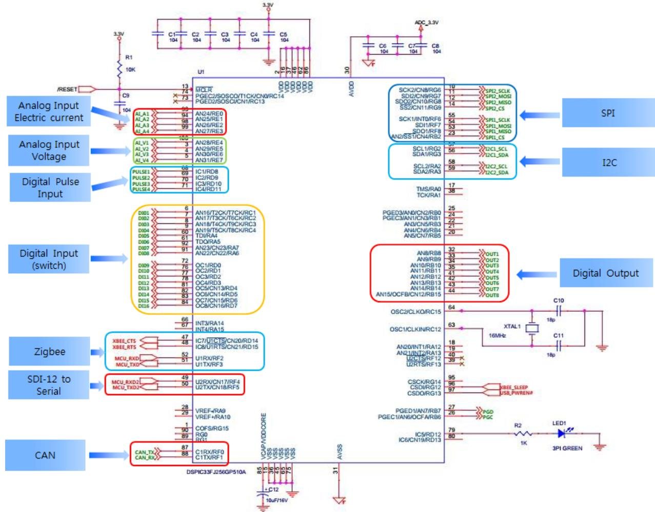
Figure 1. Circuit diagram of the MCU part (MICROCHIP, dsPIC33FJ).
