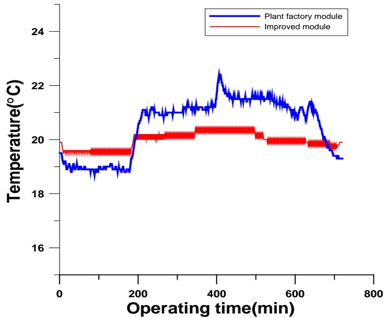
Figure 9. Results of measurement the temperature in plant factory.
