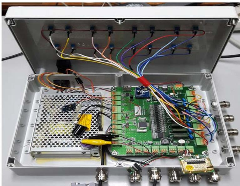
Figure 8. Internal structure of the fabricated sensor and actuator interface module.
