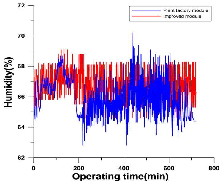
Figure 10. Results of measurement the humidity in plant factory
