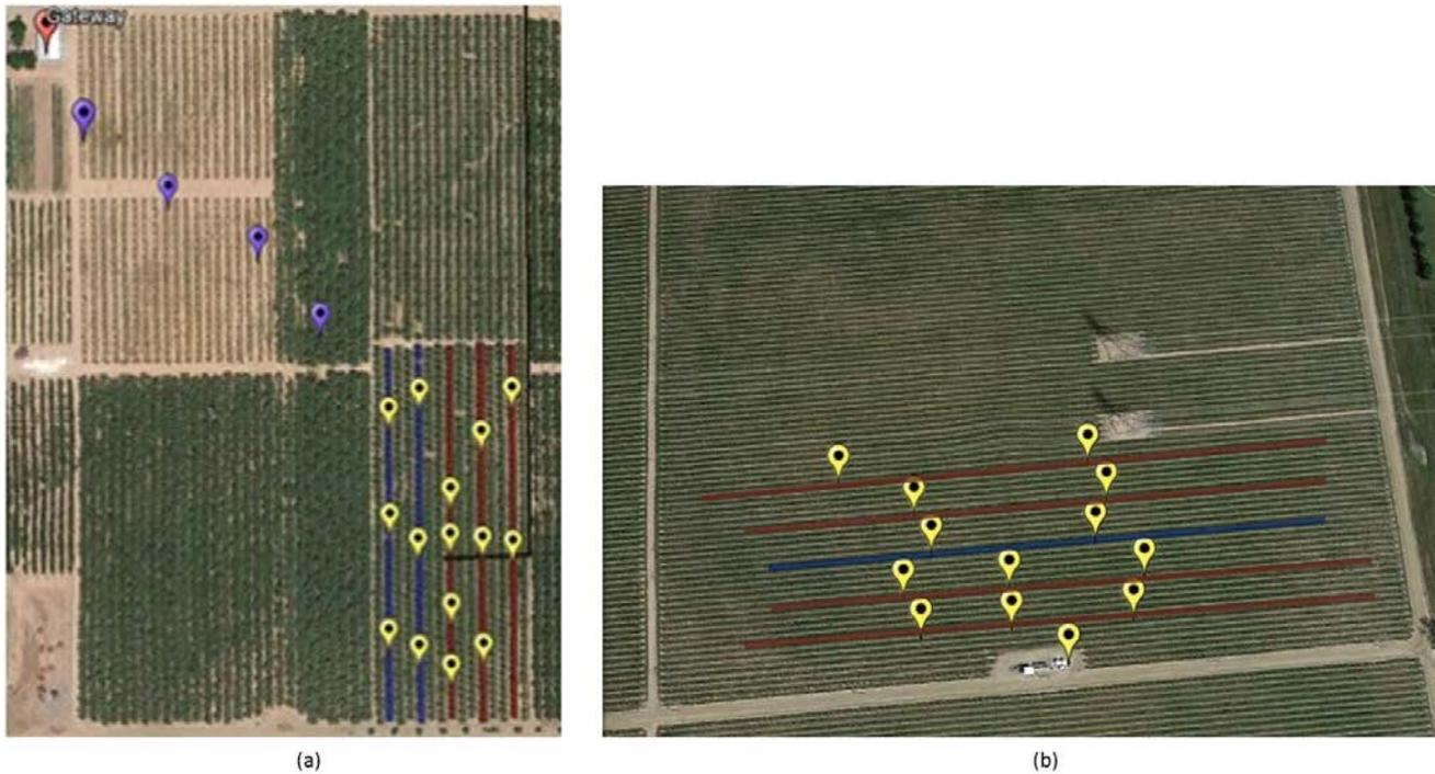
**Fig. 2 Google Earth images of (a) node locations (yellow), repeater locations (blue), and gateway location (red) in almonds and (b) hub locations in grapes. In each, blue rows indicate grower treatment and red lines indicate PWS-based treatment**
