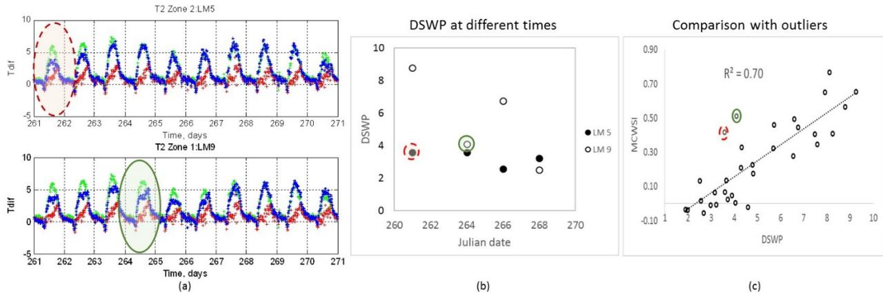
**Fig. 8** Outlier analysis of (a) temperature difference plots over time (in Julian days) as vines recover from a period of water stress for leaf monitor #5 (top) and leaf monitor #9 (bottom); (b) DSWP over time as measured with a pressure chamber for leaf monitor #9 (open circles) and for leaf monitor #5 (closed circles); (c) DSWP values compared with MCWSI measurements obtained from leaf monitors yielded an  $R^2$  value of 0.70 with suspected outliers
