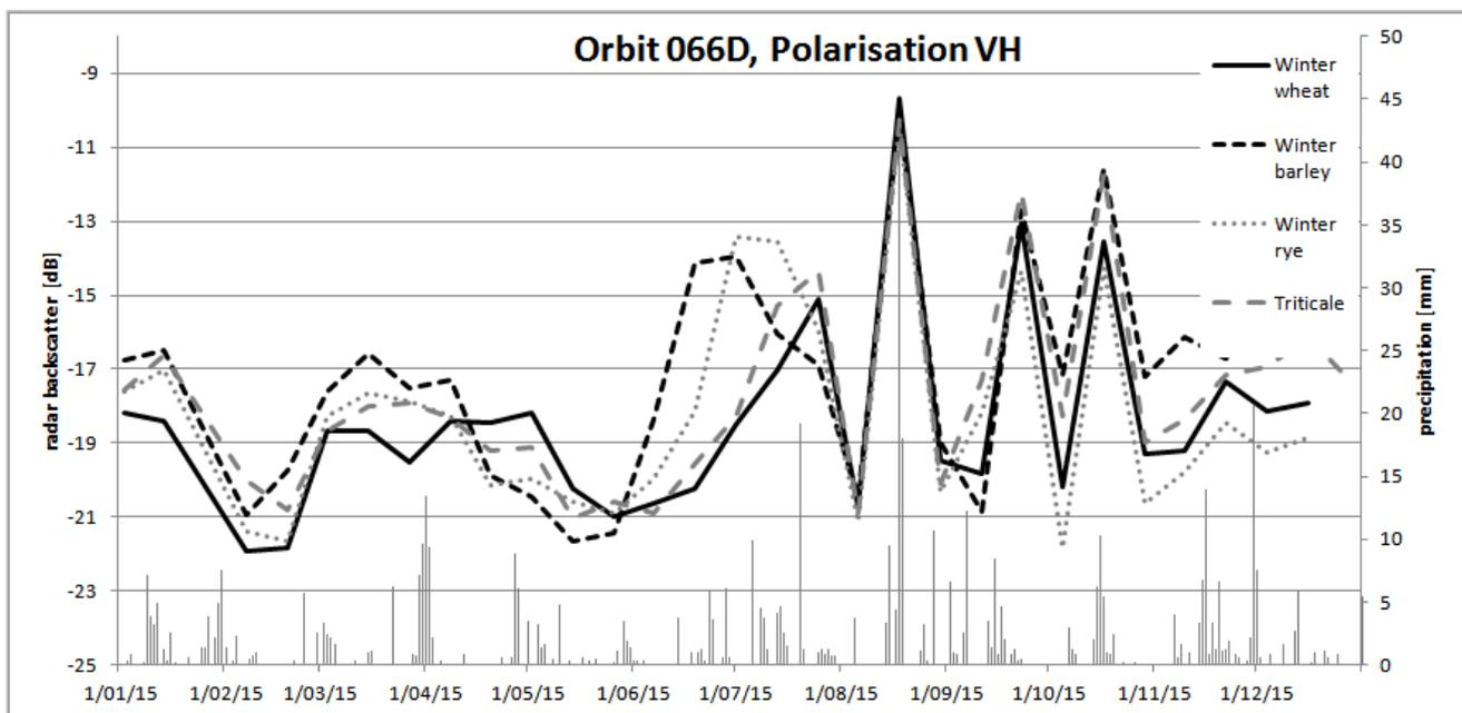
Fig 3. Radar backscatter signatures of Sentinel-1A for different cereals overlaid with daily precipitation data of weather station Helmstedt (B).
