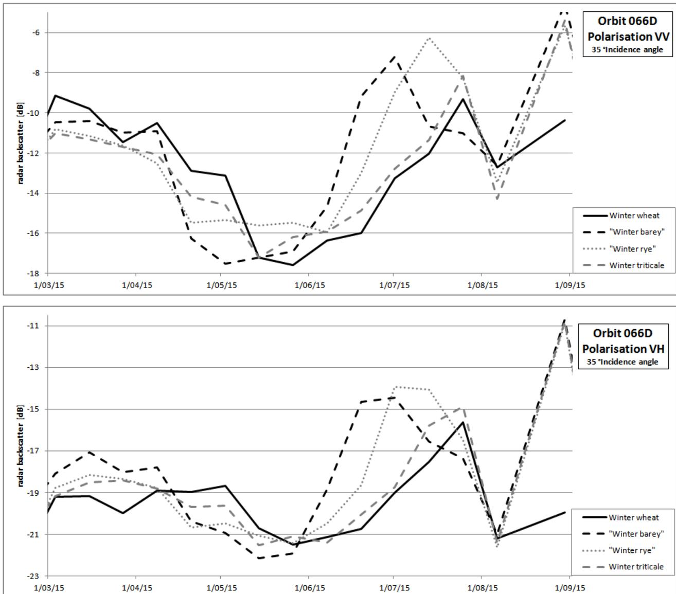
Fig 4. Radar backscatter signatures for cereals, top: co-polarization, bottom: cross polarization.
