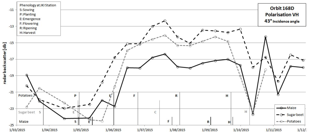
Fig 6. Radar backscatter signatures for maize, sugar beet and potatoes at 43° incidence angle, and phenological dates of the crops at the JKI research station.
