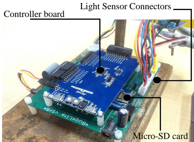
Figure 1. Prototype for main controller board
