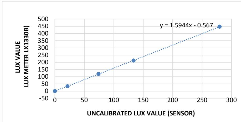
Figure 5. Calibration equation using linear regression
