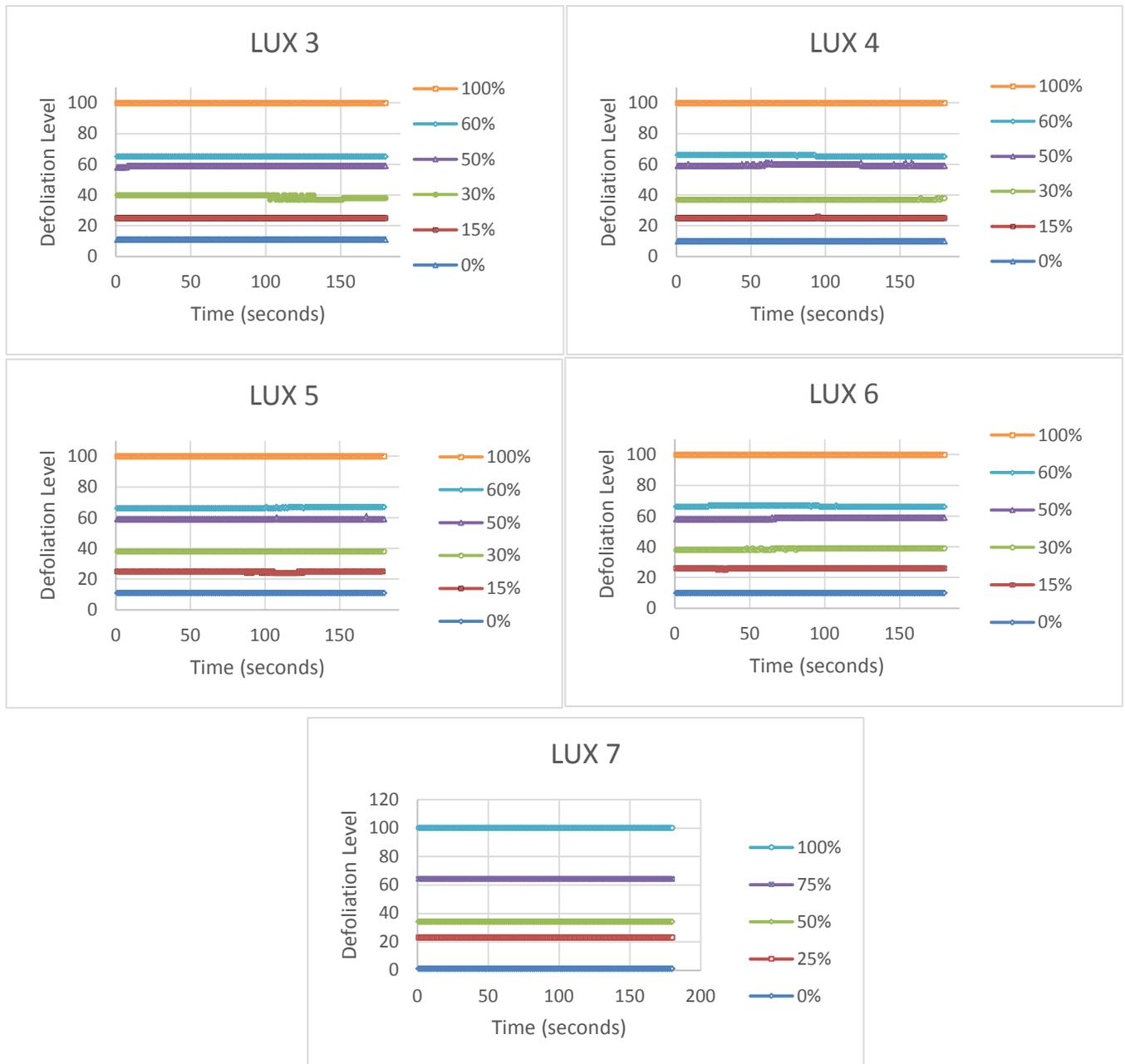
**Figure 9.** Estimates of defoliation from the first defoliation sensor to filter paper covers with varying levels of simulated defoliation at light intensities  $lux_3$  to  $lux_7$ .
