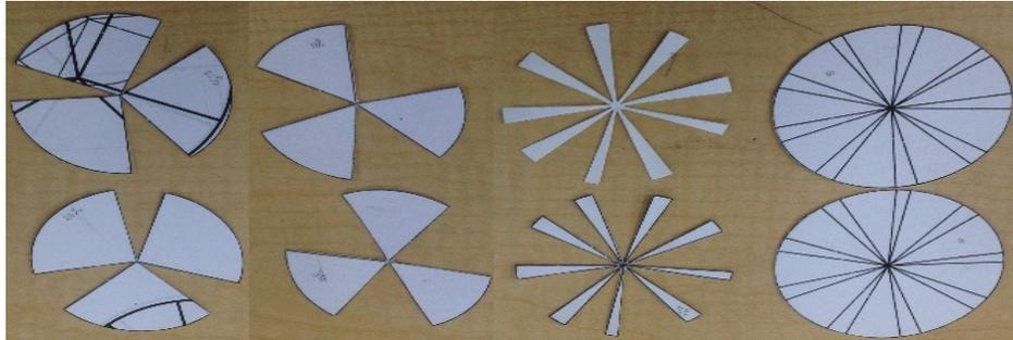
**Figure 3. Simulated defoliation levels of 25, 50, 75, and 0 (left to right) to cardstock covers for testing defoliation sensor.**
