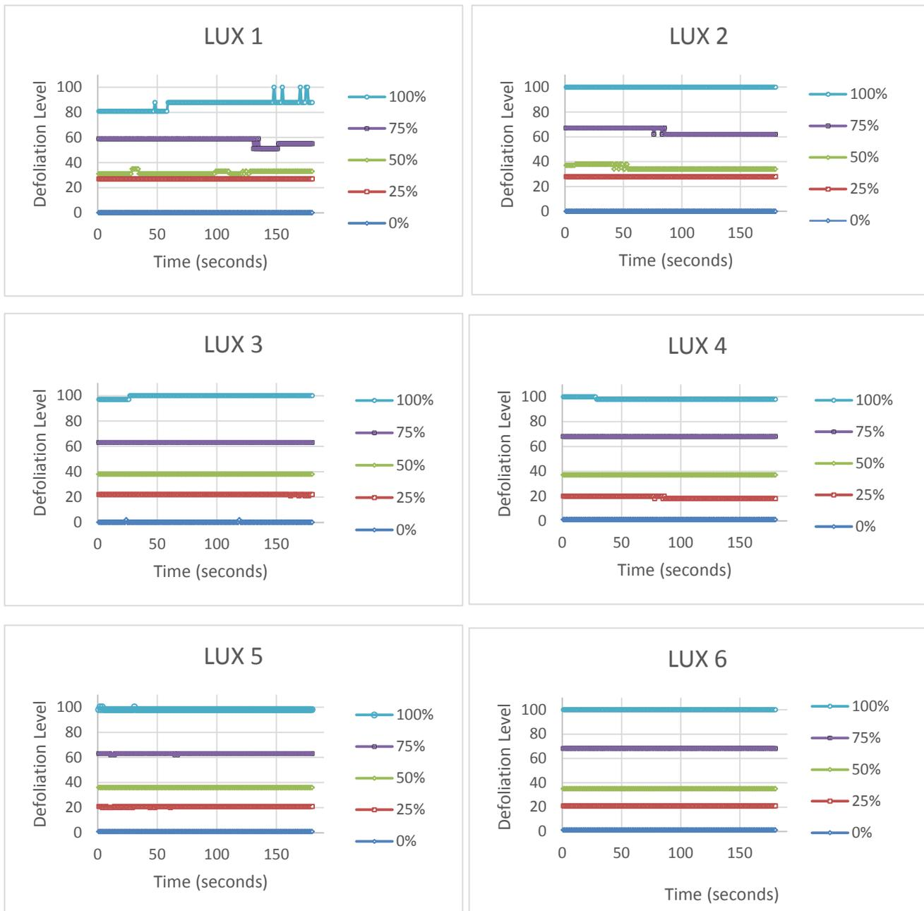
**Figure 6. Estimates of defoliation from the first defoliation sensor to cardstock covers with varying levels of simulated defoliation at light intensities  $lux_1$  to  $lux_7$ .**
