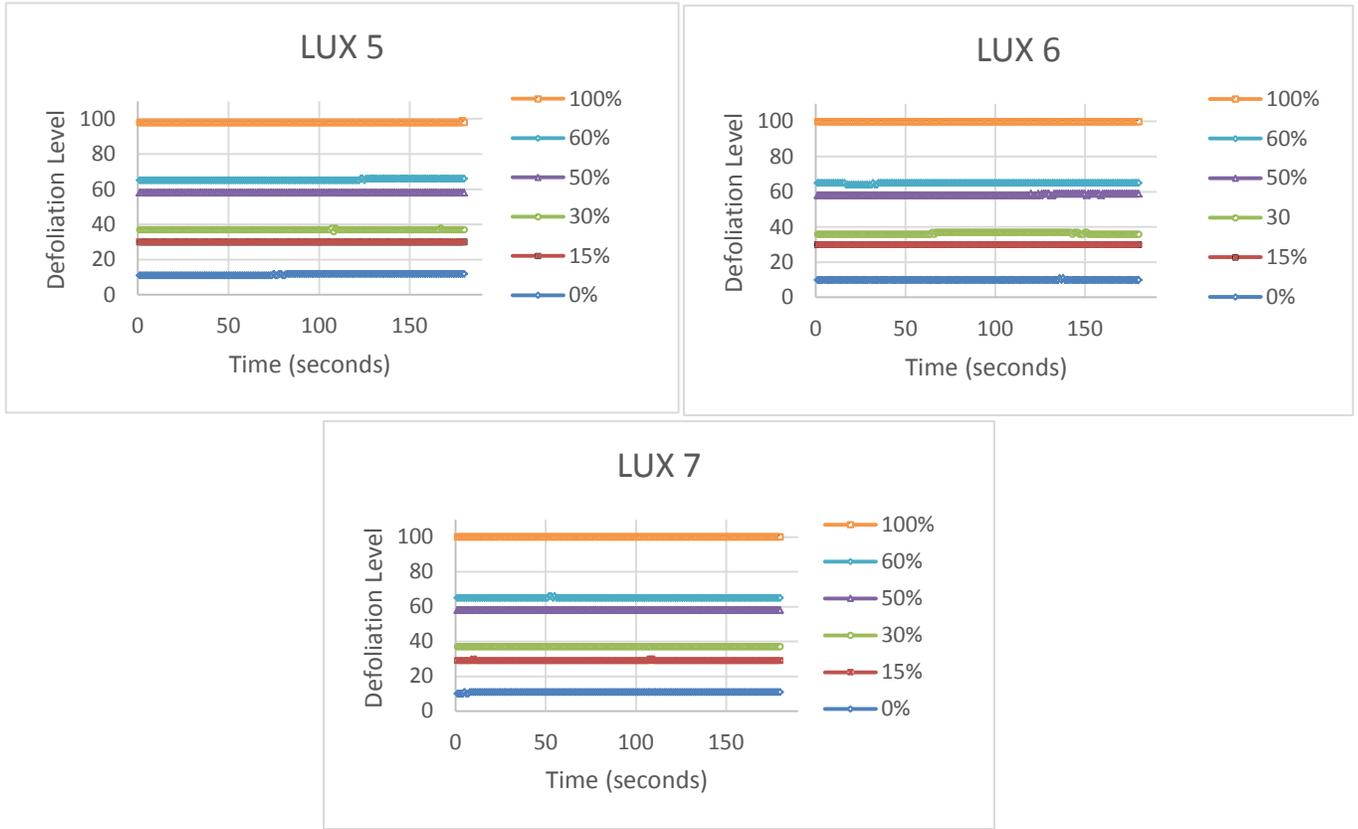
Figure 10. Estimates of defoliation from the second defoliation sensor to filter paper covers with varying levels of simulated defoliation at light intensities  $lux_3$  to  $lux_7$ .
