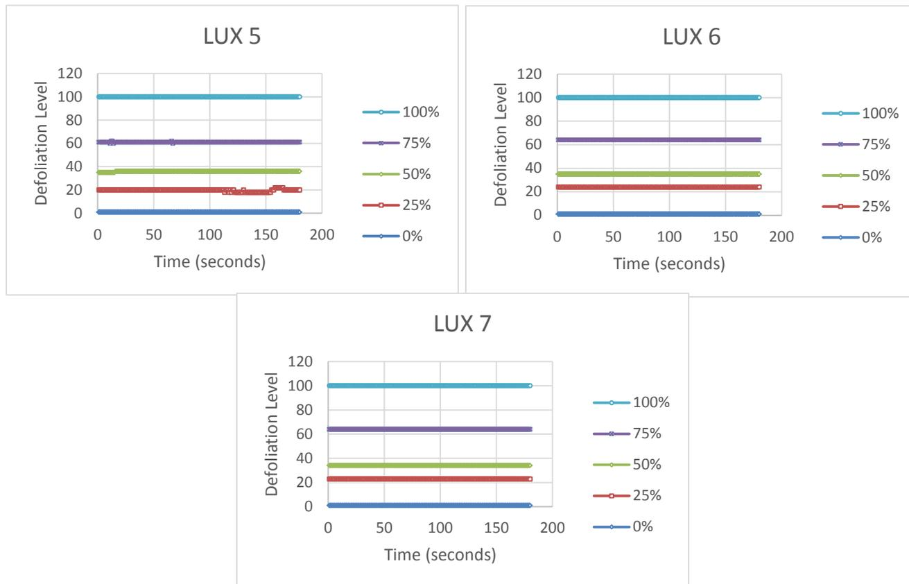
Figure 7. Estimates of defoliation from the second defoliation sensor to cardstock covers with varying levels of simulated defoliation at light intensities  $lux_1$  to  $lux_7$ .
