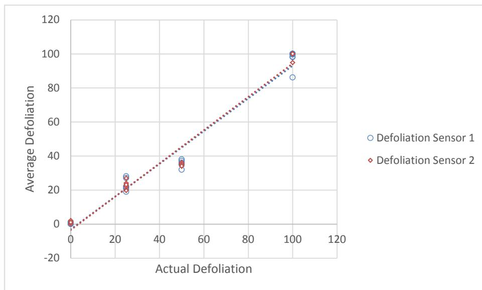
Figure 8. Linear regression line of defoliation accuracy resulting from first defoliation sensor with slope and  $R^2$  equal to 0.9609 and 0.969 respectively and second defoliation sensor with slope and  $R^2$  equal to 0.9779 and 0.9696 respectively.
