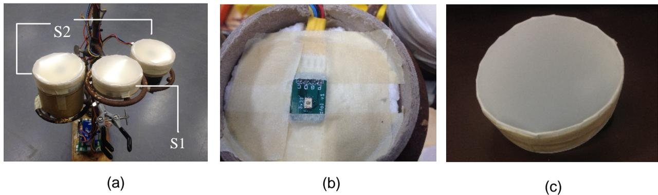
Figure 2. Setup of (a) defoliation sensor module is composed of (b) light sensor and (c) diffuser film.
