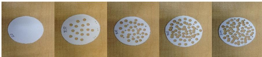
**Figure 4. Simulated defoliation Level 0, 15, 30, 50 and 60 (left to right) to filter paper for testing defoliation sensor.**
