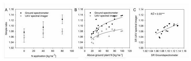
Fig 7. The spectral N status indicator Simple Ratio (SR) as affected by N application (A) and Total N in the above ground biomass (B) shown for the ground and UAV based spectral measurements. The relationship between the ground based spectrometer and UAV spectral measurements is shown in (C).
