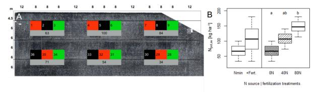
Fig. 3. A randomized field trial with six plot replicates (6 x 8 m) marked with colors (A). The three N input treatments: 0, 40 or 80 kg N/ha are shown in black, green and red, respectively. Soil available N determined prior to seeding by the Nminmethod for each block is shown in the grey bar below. Potentially available N as affected by the soil N stock or fertilization treatment is shown in (B)
