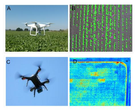
Fig. 4. A commercial quadrocopter used for RGB image acquisition (A) for development of weed detection algorithms (B); another commercially available quadrotor platform mounted with a Gamaya camera system (C) and a derived false color map indicating N status in sugar beet (D).
