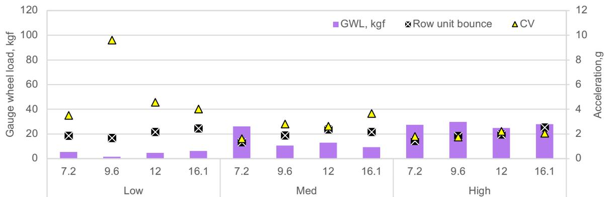
Figure 8. The response of row unit bounce at fixed downforce setting with increasing ground speed at 6.35 cm (2in) target seeding depth
