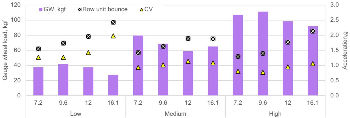
Figure 7. The response of row unit bounce at fixed downforce setting with increasing ground speed
