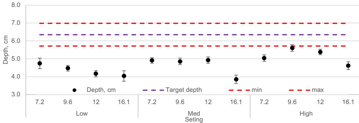
**Figure 5. Average seeding depth for the fixed downforce setting across different ground speeds at 6.35 cm (2.5 in) target seeding depth**
