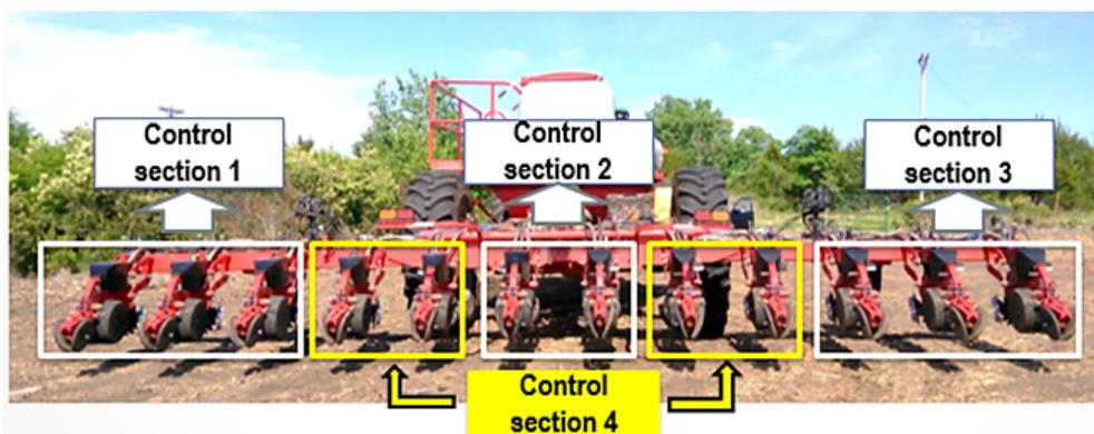
Figure 1. The planter toolbar segregated into 4 different control sections.
