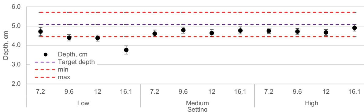
**Figure 4. Average seeding depth for the fixed downforce setting at different ground speed**
