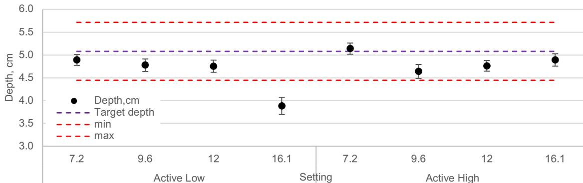
**Figure 6. Average seeding depth for the active downforce setting at different ground speed**
