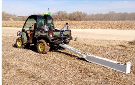
Figure 3. The DualEM-1S electromagnetic induction sensor used to collect soil EC<sub>a</sub>
