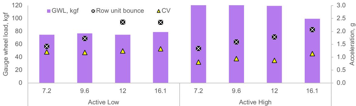
Figure 9. The response of row unit bounce at fixed downforce setting with increasing ground speed
