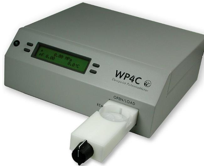
Fig 11. WPC4 water potential meter from Decagon.
