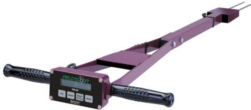
Fig 2. TDR soil moisture sensor.
