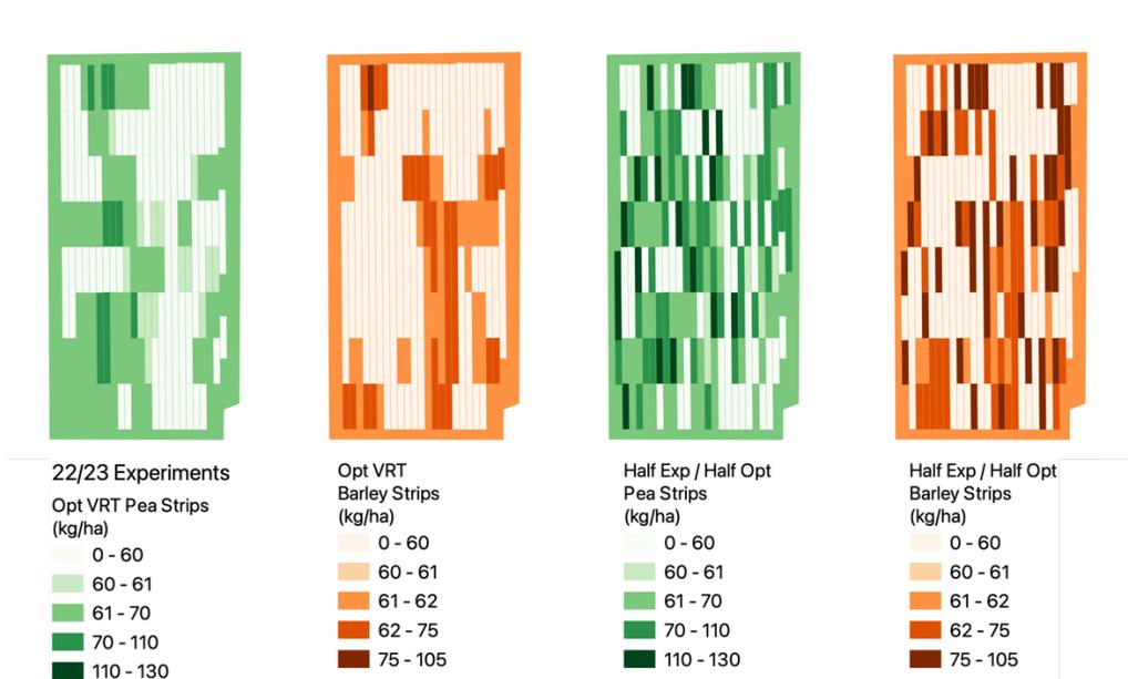
**Figure 7D) 32 hectare Field A showing optimum variable rates given actual seeder capabilities in width (21m) and length given speed of variable rate change (73m); panel 1) optimum variable pea rates, 2) optimum variable barley rates, and in panels 3 and 4) half the strips are randomized for continued experimentation. These are the rates we would recommend for the farmer the following seasons this rotation repeats.**
