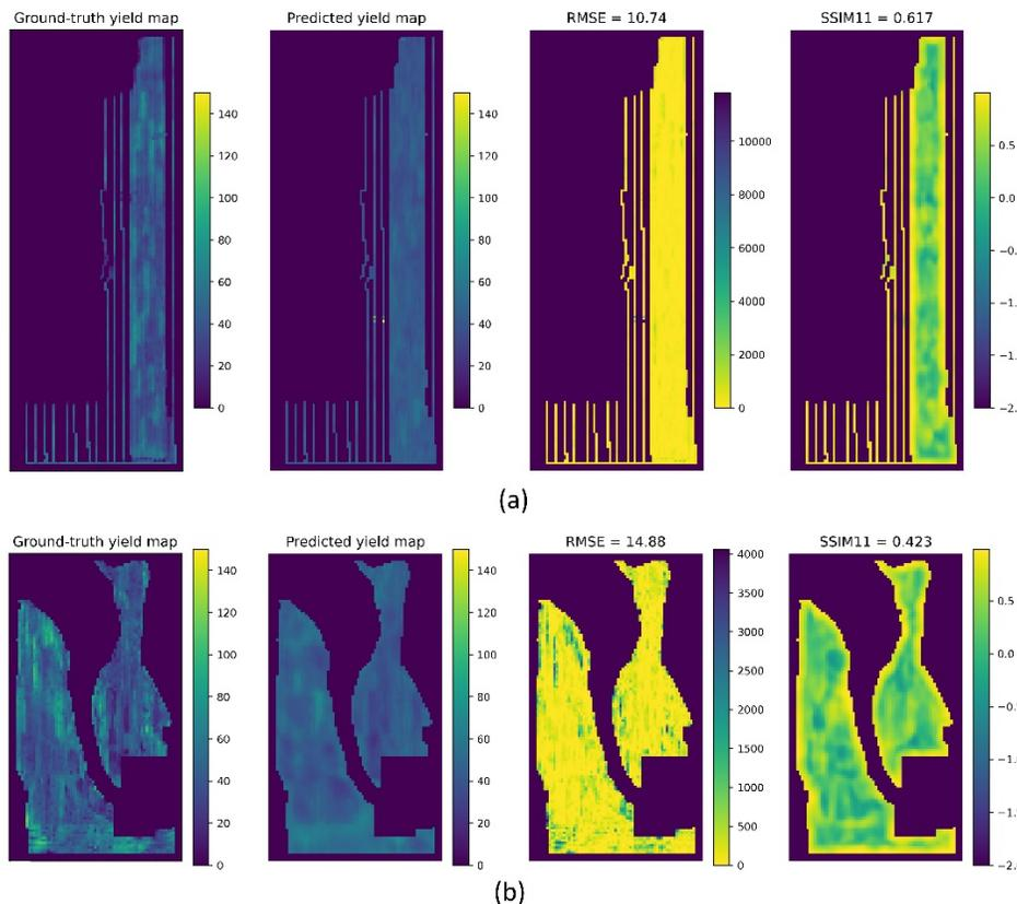
Fig 3. Yield prediction, square error map, and structural similarity map of the (a) F1 field and (b) G1 field.
