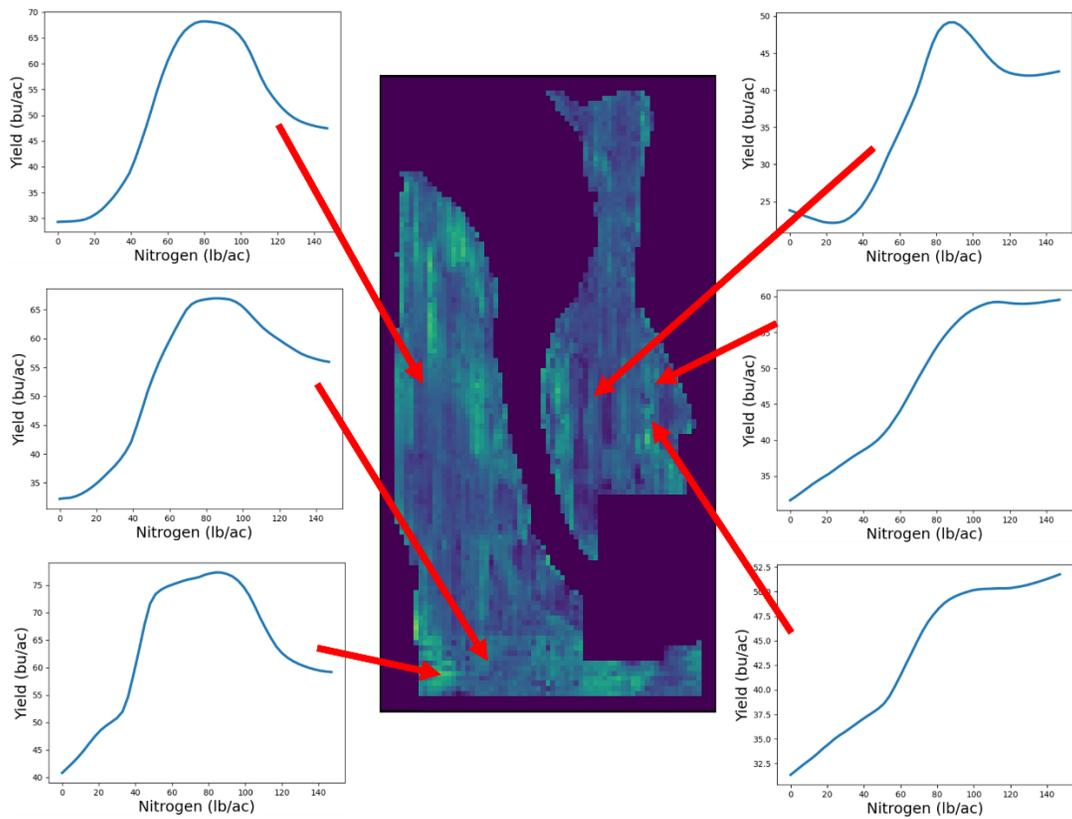
Fig 6. N-response curves generated for different regions of the G1 field.
