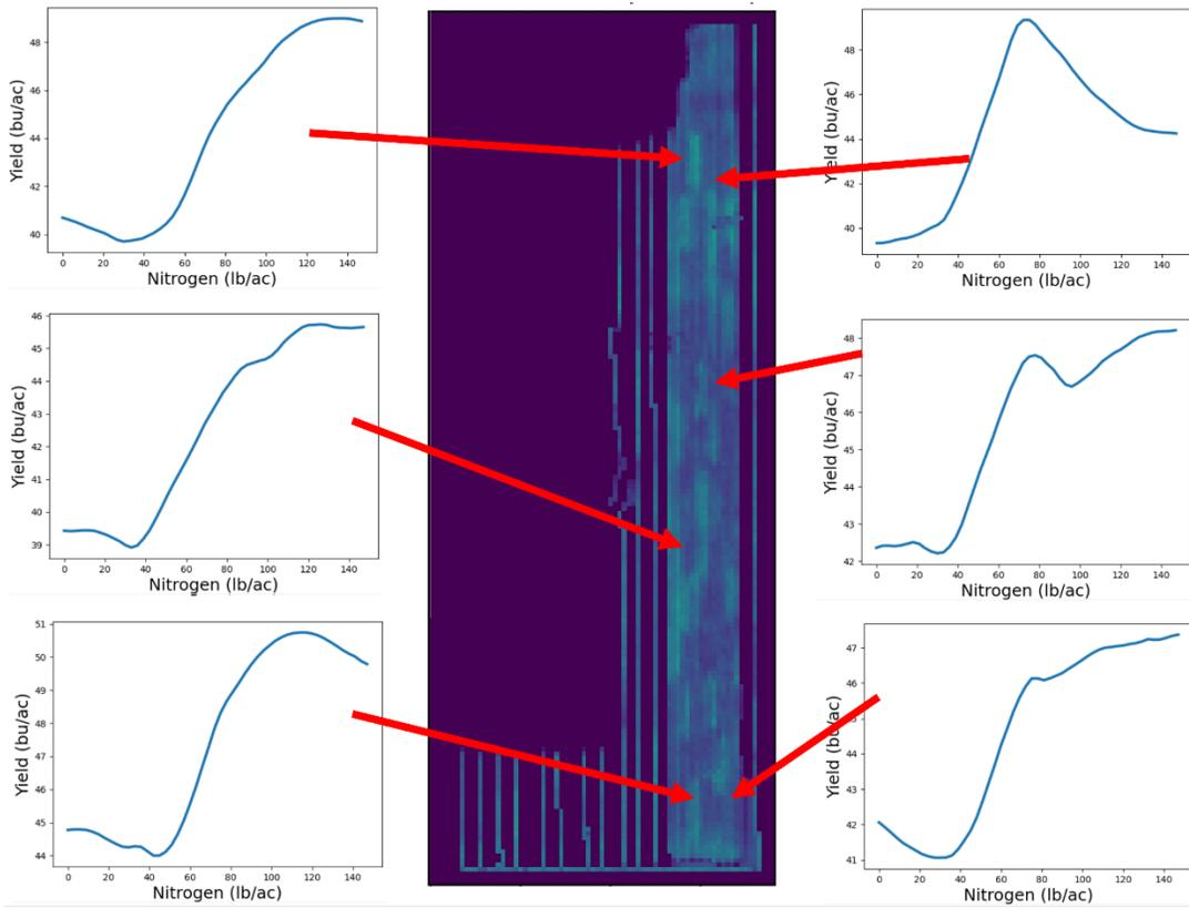
Fig 5. N-response curves generated for different regions of the F1 field.
