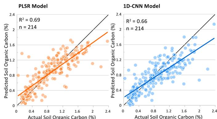
Figure 1: Testing model results of predicting soil organic carbon using VNIR with a PLSR and 1D-CNN.
