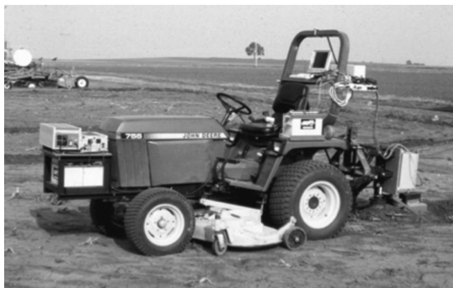
FIGURE 1.7 Soil organic matter sensor based on NIR reflectance. (From Sudduth, K. A. et al., Soil organic matter sensing: A developing science. In: G. A. Kranzler (ed.), Automated Agriculture for the 21st Century . ASAE Publication 11-91, St. Joseph, MI, pp. 307-316, 1991.)
