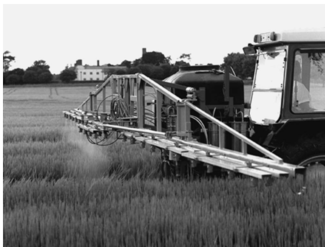
FIGURE 1.5 Variable rate herbicide applicator developed by Stafford and Miller (1993).
