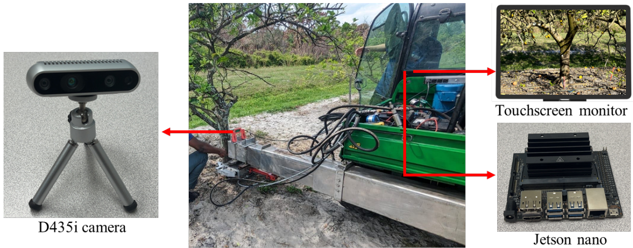
Fig. 3. Field testing of the 3-D vision sensing system in a citrus grove.
