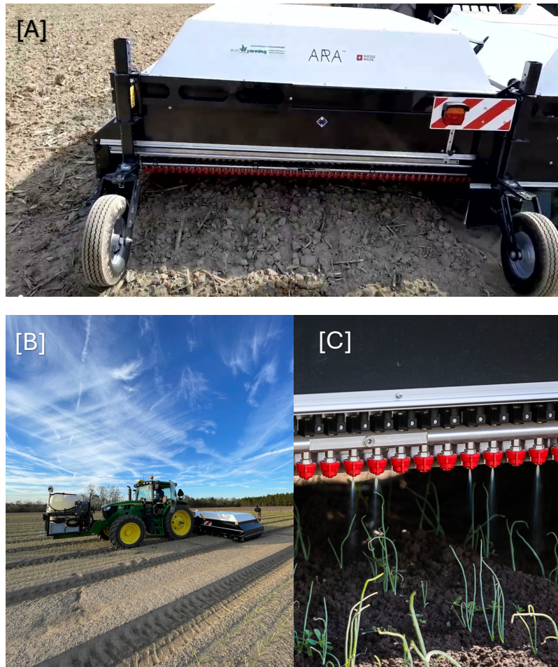
Figure 2: Left-side view of the Ecorobotix ARA system showing the spraying unit [A]; Overview of the Ecorobotix ARA system operating in the onion field [B]; C: Detail of the high-frequency nozzles used for targeted application [C]
