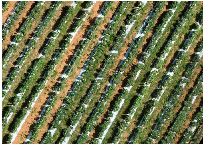
Figure 7: Orthomosaic of the tomato experimental area obtained from aerial images acquired at a flight altitude of 40 m.
