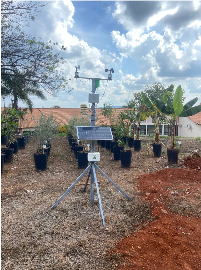
Fig. 1 Inova Precisão station at EPAMIG ITAP during 31-day validation alongside Davis Vantage Pro2
