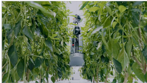
Fig. 7 Sweet pepper harvesting robot "L"
