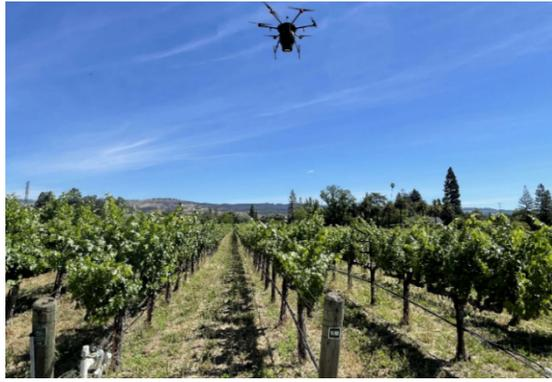
Fig 2. Hyperspectral data collection of the vineyard from the UAV.
