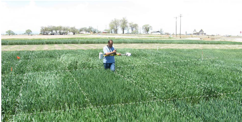
Figure 1. Collecting NDVI readings using Greenseeker ® hand held optical sensor. Plot boundaries are highlighted with dashed lines.
