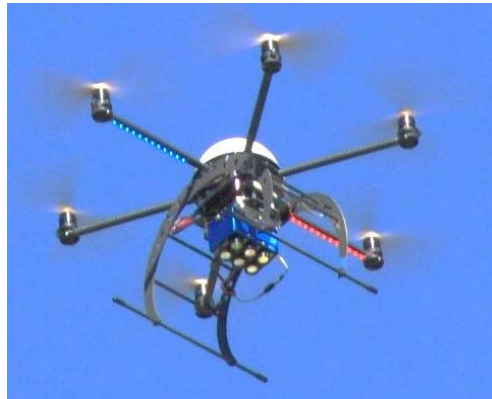
Figure 1. Multi-rotor remote sensing platform with six-band sensor.
