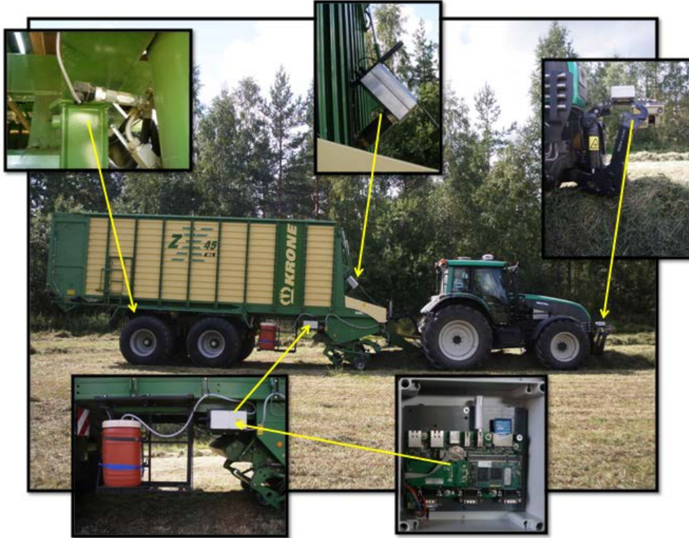
Figure 2. The tractor–loader wagon combination with additional devices: pressure sensor, NIR, laser scanner, additive applicator, and additive applicator ECU.
