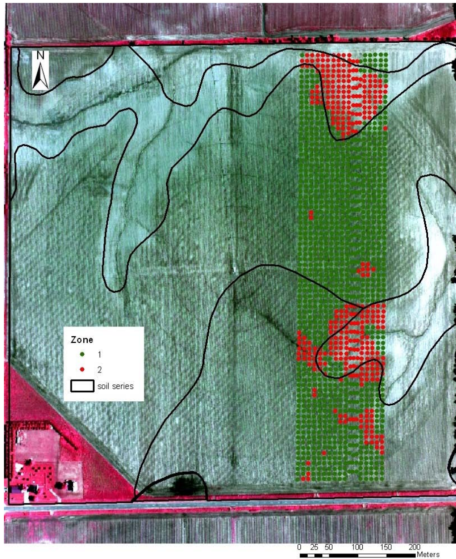
Fig. 2. Zones 1 and 2 resulting from MZA clustering of soil variables. Data points and soil series are overlaid on a bare soil CIR image.
