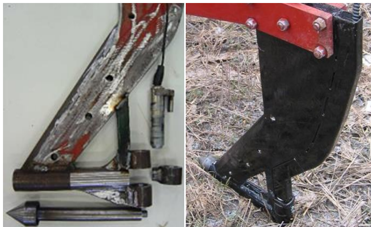
Figure 1. Detailed picture of the horizontal penetrometer and its components.
