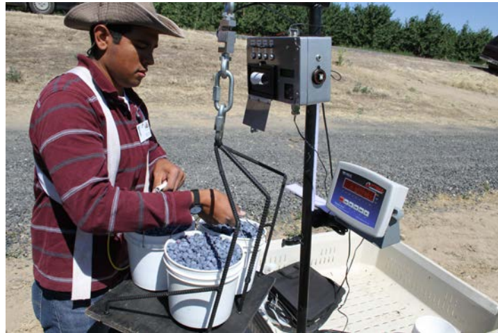
Figure 5. A blueberry picker places his buckets on the suspended platform, initiates the weighing system with his RFID-wristband by passing it before the reader, and collects the receipt.
