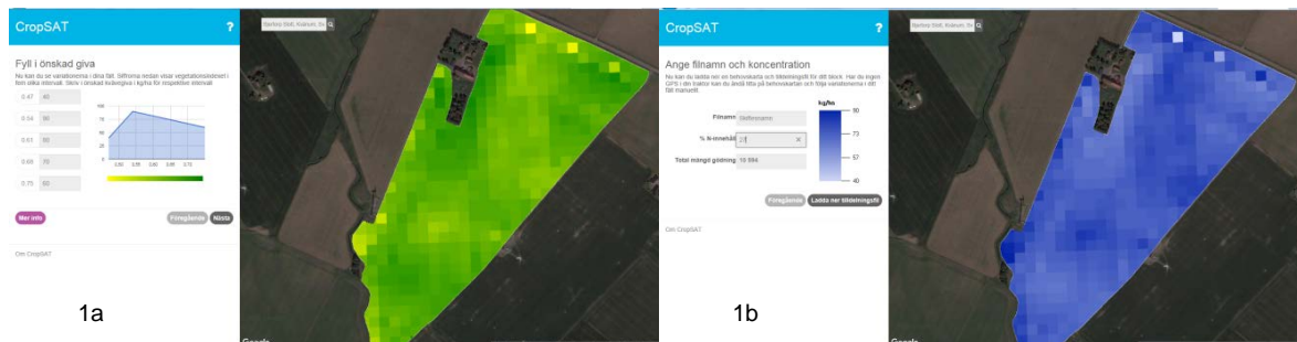
Figure 1 a) Vegetation index displayed on Google Maps, where the user must enter five levels of N fertilization compared with the colored scale. b) A VRA file ready to be entered into the fertilizer spreader via a USB memory stick.
