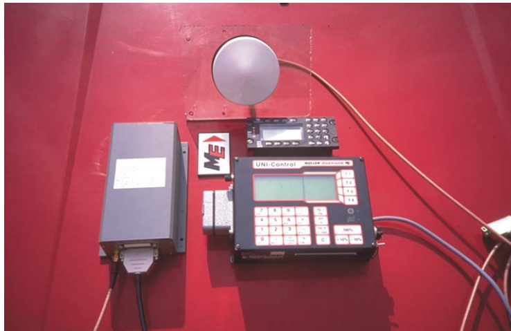
Fig 1. First GPS system and bord computer employed in agriculture in Germany
