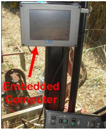
Fig. 2. Embedded computer located inside the cabin of harvester.
