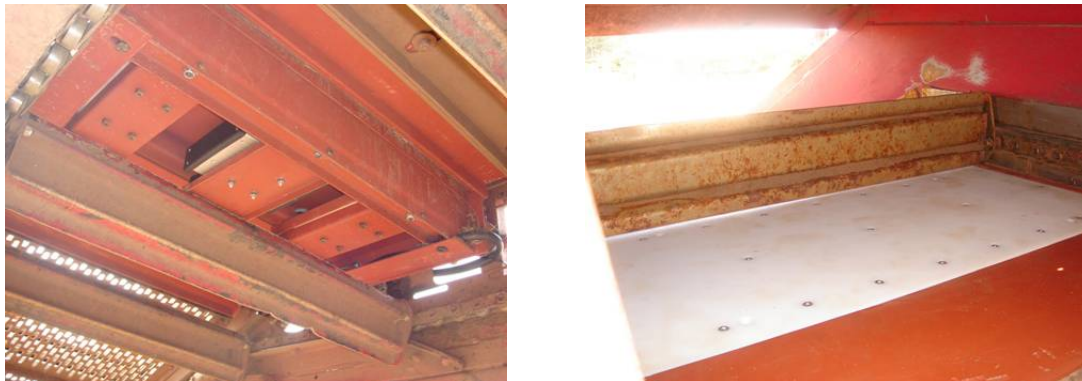
Fig. 3. Weighing system installed on the harvester.
