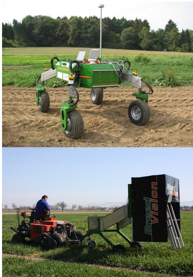
Fig. 11 Phenotyping platforms: Autonomous field robot BoniRob (top) and tractor-mounted platform BreedVision (bottom).
