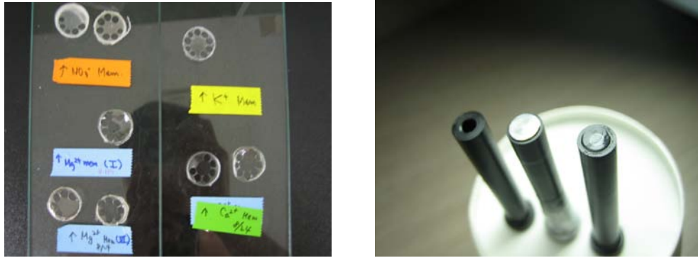
Fig. 1. Ion-selective membranes for N, K, Ca, and Mg (left) and cobalt electrode for P (right).
