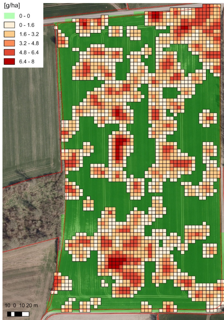
Figure 3 The variable Lexus 50 WG shapefile for case 4 to be imported in the sprayer terminal
