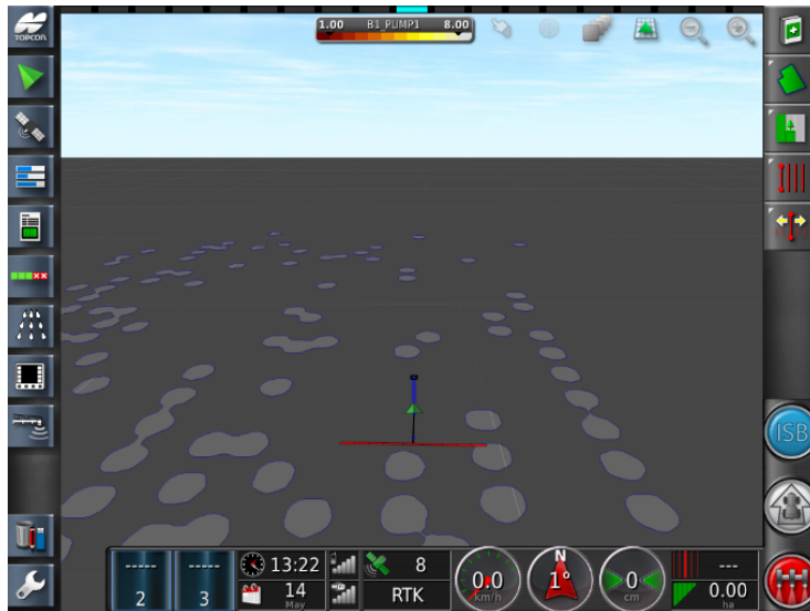
Figure 2 The on/off application map for the DFF herbicide case 3 imported into the Topcon X35 terminal
