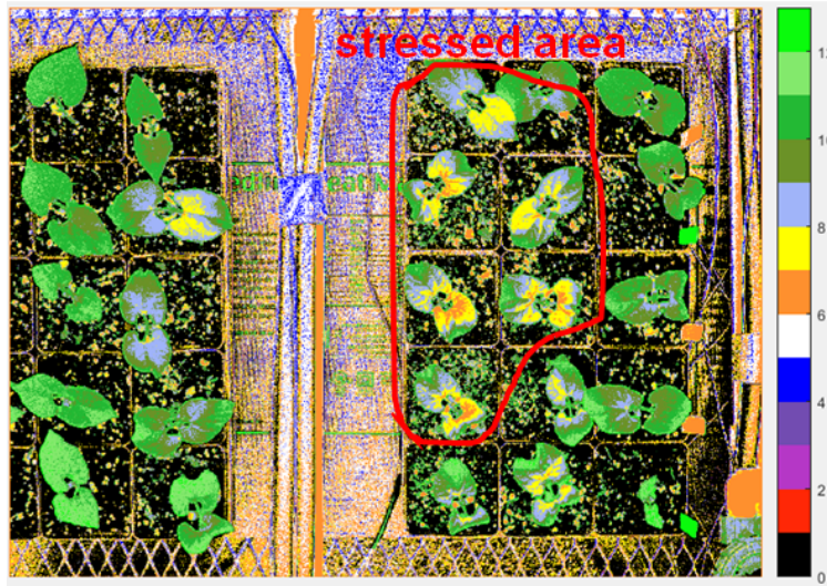
Fig 5. One NDVI map calculated from one image taken in our greenhouse experiment. The color bar on far right shows the range of NDVI indices. Higher NDVI indices (i.e. 12) indicate healthier vegetation. As we can see, the plants near the center of the figure (circled by red) are less healthy than the other plants.
