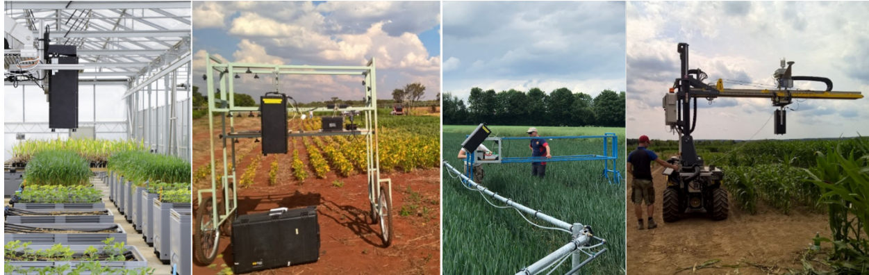
Fig 2. Light Induced Fluorescence Transient (LIFT) instrument (black rectangular camera) integrated in different positioning platforms from left to right measuring various crops in the miniplots, in the field in soybean Embrapa, Brazil, in wheat BreedFACE, Germany and with the field cop measuring maize in the common experiment in Germany,
