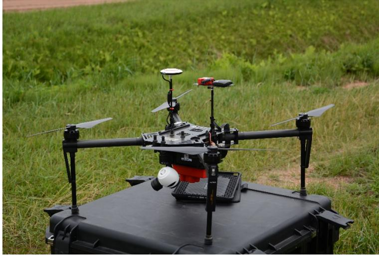
**Figure 4. DJI Matrice 100 equipped with multi-spectral camera and visible light camera used for data acquisition over cranberry beds. This platform also had the ability to implement thermal measurements in place of the visible light camera.**
