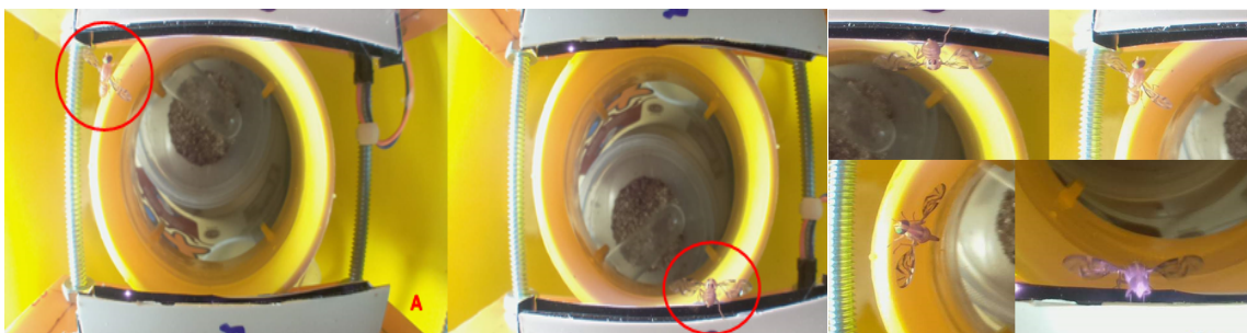
Figure 7 - Images captured when different flies pass through the optoelectronic sensor.
