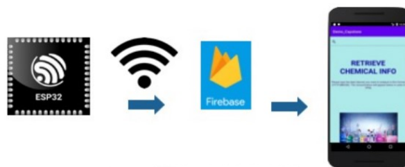
Figure 9: Overall connection diagram of dataflow from the spectrophotometer to the Android application
