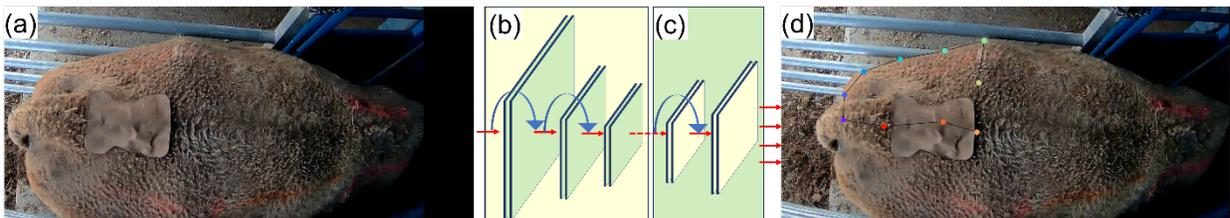
Fig 3. The diagram outlines the DeepLabCut pose estimation workflow: (a) input, (b) pre-trained model (ResNet50), (c) deconvolutional layers, and (d) output with pose skeleton.
