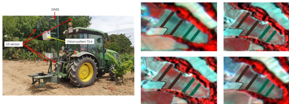
Figure 6. Developed device provided with ultrasonic sensors for in-field canopy measurements (right); results obtained after in-field measurements compared with satellite images in order to determine the optimal relationship (left).
