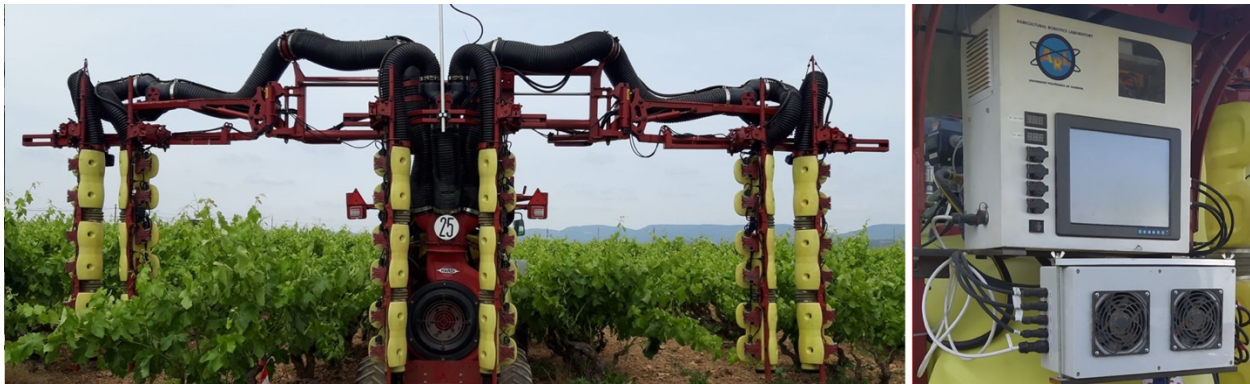
Figure 4. General image of the smart multi-row sprayer for vineyards during an application (left) and detail of the computer for map interpretation and spray control.
