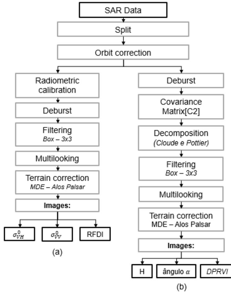
Fig. 3 - Processing flow of SAR images for backscatter coefficient data (a) and for polarimetric decomposition (b).
