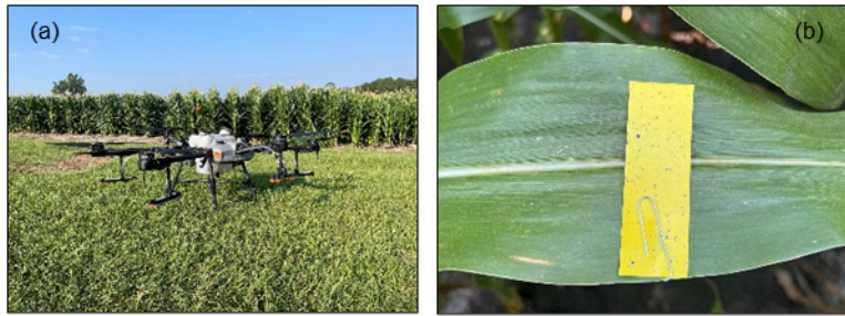
Figure 1: (a) The DJI Agras T40 Spray Drone and (b) a water-sensitive paper attached to a corn leaf.
