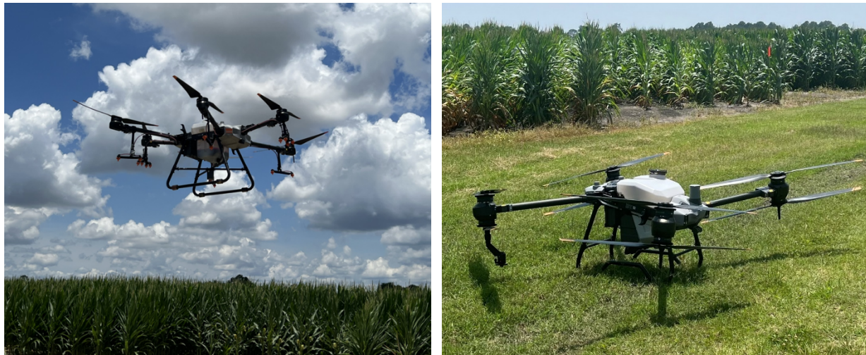
Figure 1. DJI T30 and T40 spray drones used for deposition and efficacy evaluation studies.
