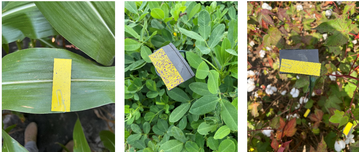
Figure 2. Illustration of water-sensitive paper placement in different crop canopies used for spray deposition assessment in the studies conducted in 2023.
