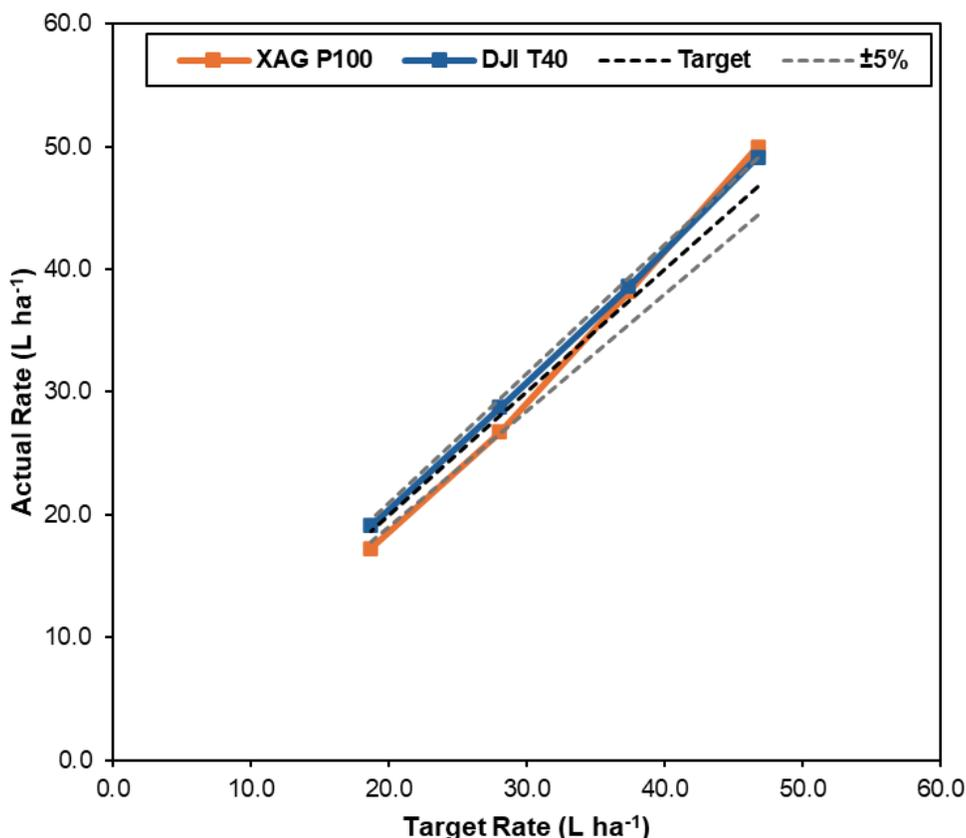
**Fig 6. Graphical representation of the actual rate (dark solid lines) versus the target application rate (black dashed line) during field testing.**
