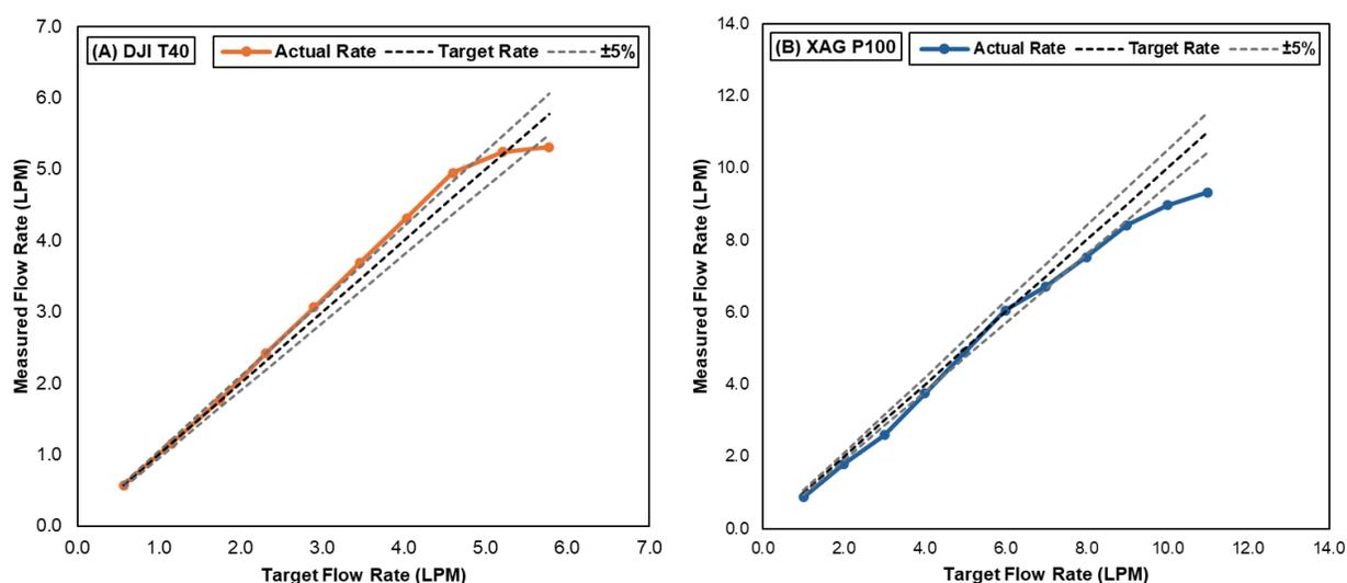
Fig 5. Graphical representation of the actual rate (dark solid lines) versus the target flow rate (black dashed line) during static testing.
