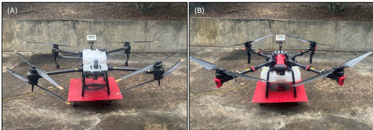
Fig 4. Illustration of weight measurement using a precision scale for the (A) DJI Agras T40 and (B) XAG P100 Pro.
