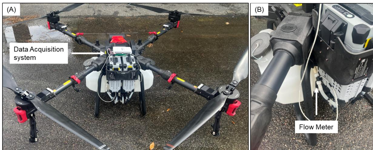
Fig 1. (A) NI USB-6210 DAQ. (B) A Flow meter was installed to measure flow rate.
