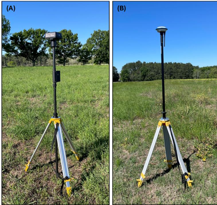
Fig 3. (A) D-RTK 2 High Precision GNSS Mobile Station and (B) XAG RTK Mobile Station
