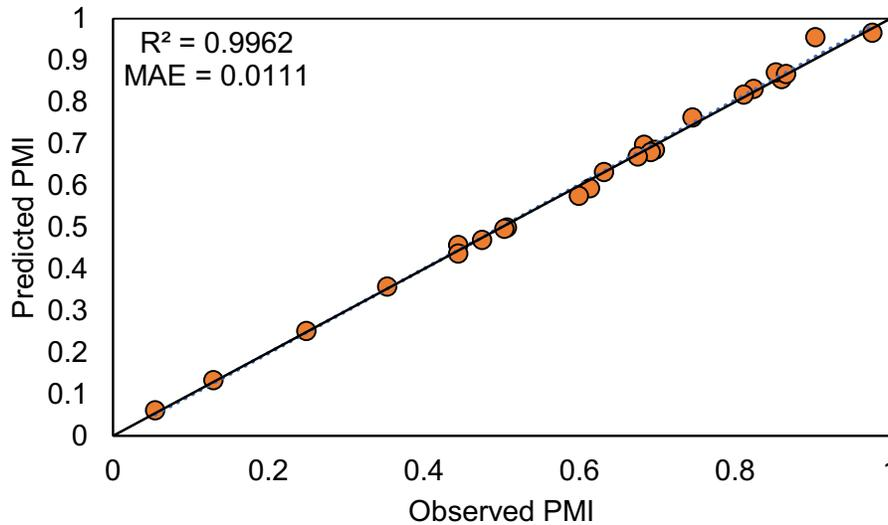
**Fig 5. Performance analysis of test dataset comparing the predicted PMI based on YOLOv9 detection and observed PMI.**
