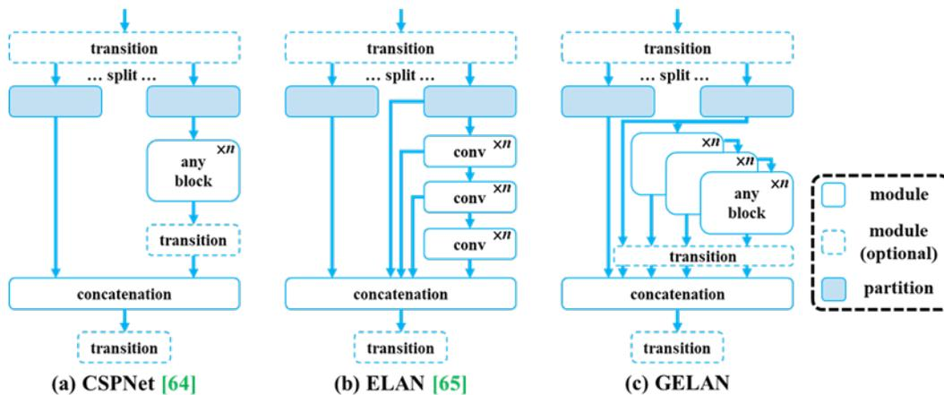
Fig 2. The architecture of GELAN within YOLOv9 (Wang et al., 2024).
