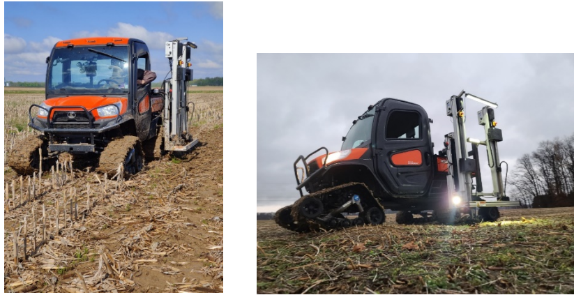
Fig 6. Dual soil cone penetrometer for data collection.
