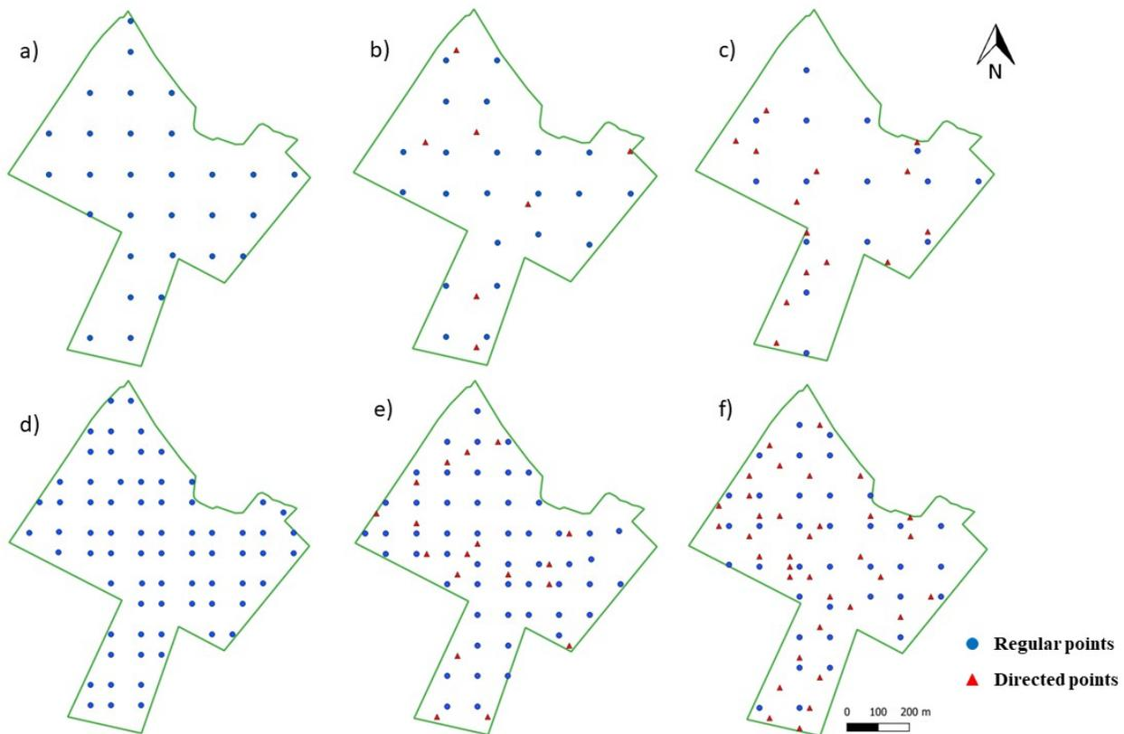
**Figure 2.** a) Regular grid 0.4 samples/ha; b) Grid with 25% of sampling points directed at 0.4 samples/ha density; c) Grid with 50% of sampling points directed at 0.4 samples/ha density; d) Regular grid 1 sample/ha; e) Grid with 25% of sampling points directed at 1 sample/ha density; f) Grid with 50% of sampling points directed at 1 sample/ha density.
