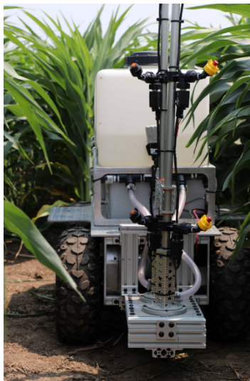
Figure 1: Robotic Sprayer System
