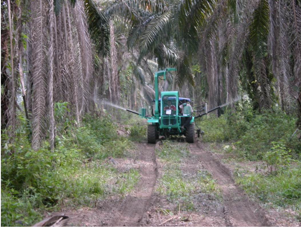
Figure 5. The VRT fertilizer applicator during fertilizer application
