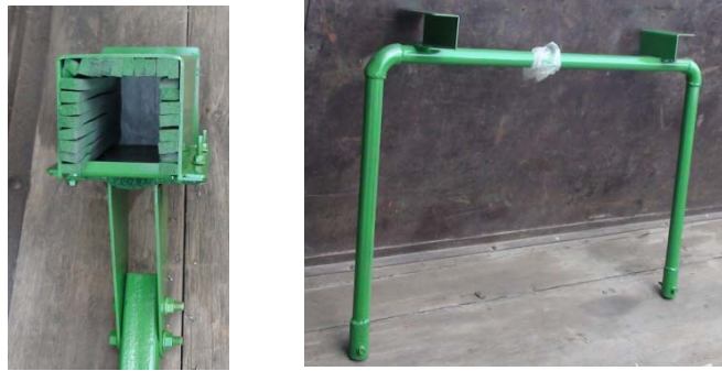
Fig. 1. Multispectral camera and N Sensor holding frame
