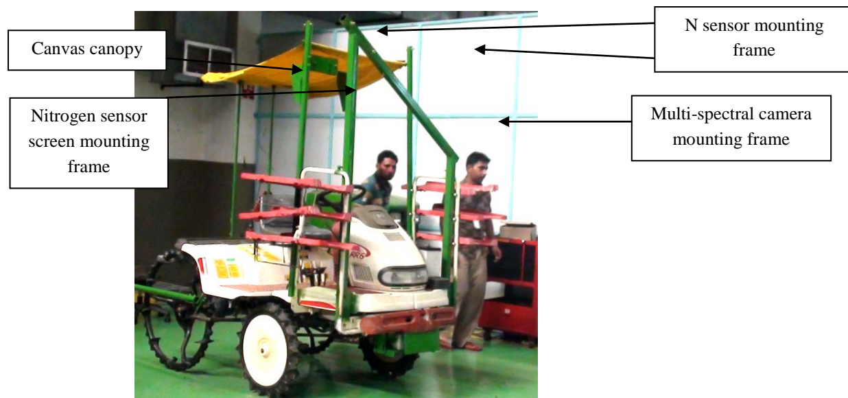
Fig. 2. Different frames mounted to the developed vehicle
