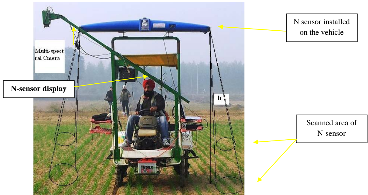
Fig. 3 View of developed vehicle with installed sensor working in the field
