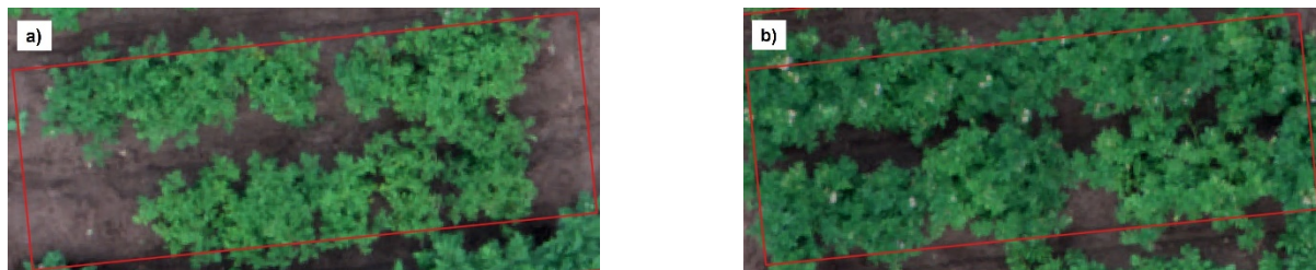
Fig. 4. Appearance of potato crops on example plots of the potato B-clones with under-estimated MC using NDRE due to a) missing plants and b) flowering plants taken into account during visual MC evaluation by the breeder but undetected by UAV imagery.
